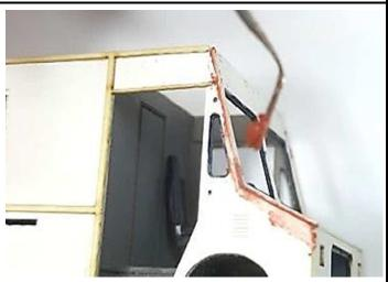
Using model or spot putty, fill any gaps in the edges of the body <u>top</u>, <u>sides</u>, <u>front and back</u>. Sand a small radius in these edges to ease the sharp corners and make the body more uniform.
