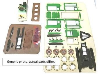
I like to paint the parts while still in the carrier. Some parts may need to be painted on the backside as well. Some touch up will be required after assembly, but this is a good start. You may not want to pre-paint really tiny parts as they may get "glued" to the carrier sheet and will be difficult to remove.
