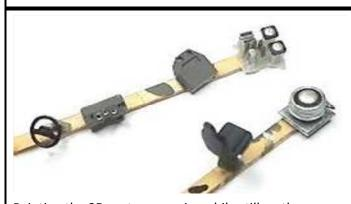
Painting the 3D parts are easier while still on the supports. I stick the parts and carrier on some double sided tape and to a popsicle stick or scrap piece of wood.
