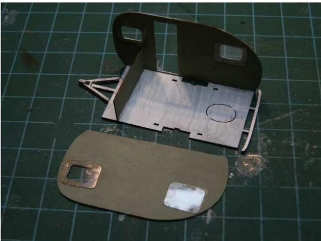
Glue one wall to the edge of the trailer frame. Then glue in the internal brace to the floor and wall.
