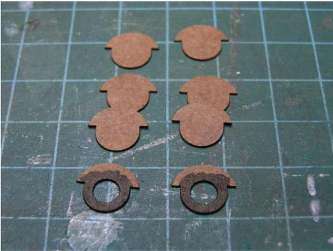
Glue and paint the 4 wheel slabs that make up each wheel.
